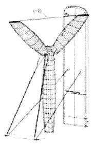
Fig. 18. Y-shaped column connected to a wall component and the pneumatic muscles (elastic tension elements).
